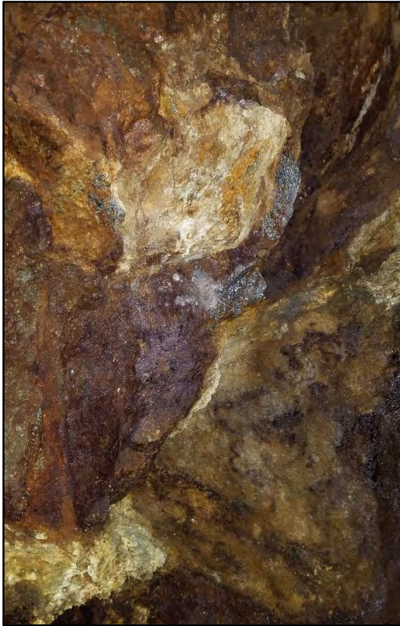
Plate 1: Sulphide Mineralization Exposed in Wall of Bleikvassli Portal; Sample M411359
